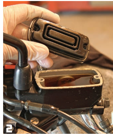
2 Remove the master cylinder cap using a Phillips head screwdriver. Make sure to cover any painted surfaces as brake fluid is very corrosive.
