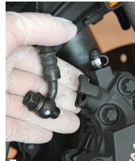
4 Using an 8mm socket remove the front brake line splitter valve from the triple tree.
