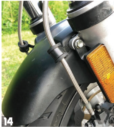
13 Tighten the new front Spiegler braided lines to each caliper using a 12mm socket.
