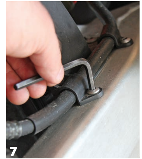
7 With a 5mm Allen remove the rear brake line guide.
