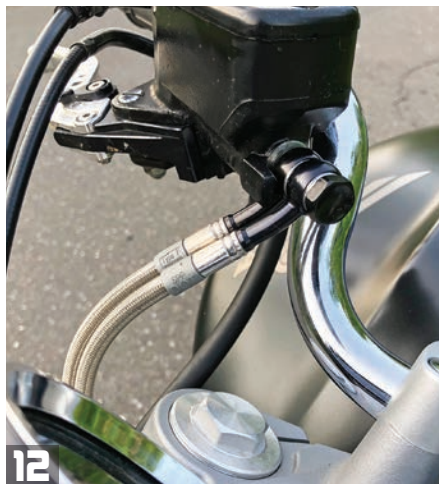
11 With the front lines I converted from the stock 1-into-2-line routing, with direct lines to each caliper. This required a new banjo bolt (provided) on the master cylinder that would accommodate two banjo fittings, one for each brake line. Provided crush washers are placed on top, bottom, and between of these fittings.
