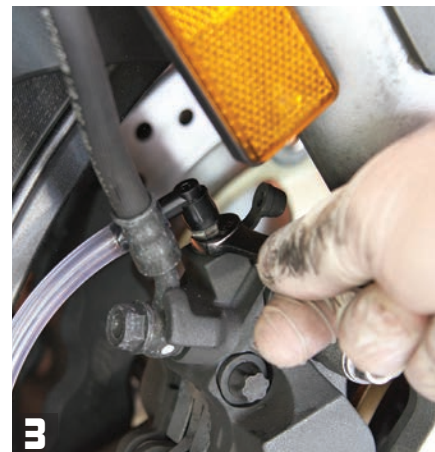
3 Locate the bleeder valve on your caliper, attach the vacuum pump tube, and loosen the bleeder valve. Then simply squeeze the pump a few times and watch the fluid flow.
