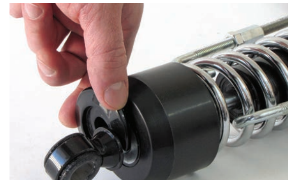
The upper spring retaining flange can be removed once the spring is compressed about 1/4".
