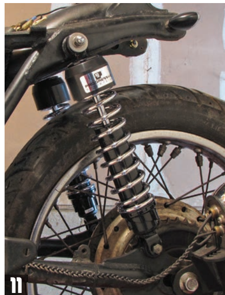
Here's a look at the new shocks installed and standing proud. GB
