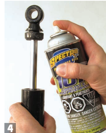
4 The bump rubber and washer may need to be lubed in order to move down the piston shaft, making room for the spring assembly.
