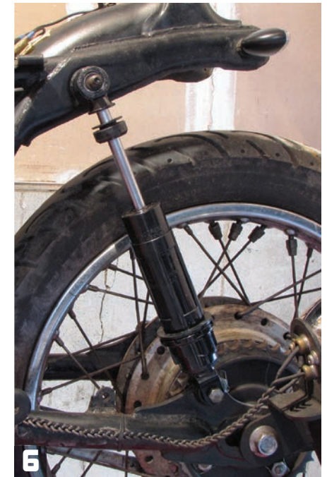
6 Install one new shock without the spring and check the clearance between the tire and fender by raising the rear wheel until the shock bottoms. There should be a minimum of 1" of clearance.
