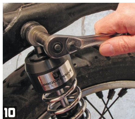
Install the new, fully assembled shocks using the original nuts and bolts, lock washers, and provided washers. A little blue Loctite can be applied to the bolts.
