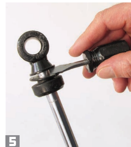
5 A flathead screwdriver assists in moving the bump rubber and washer.
