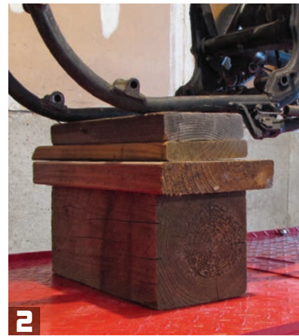
2 Prop up the rear tire to allow for adjustment when fitting the new shocks.
