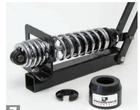
7 Assemble the springs onto the shocks using a spring compression tool. This tool will be needed and many options are available for a variety of spring and shock sizes. For this installation, we used a simple lever compression tool.
