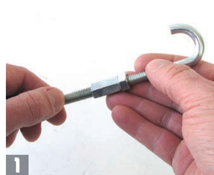
The length of angle iron bolts to the lower shock eye, and the threaded rods are connected to the J-bolts with coupling nuts. The J-bolts will pull down on the upper spring coil by tightening the coupling nuts under the angle iron.
