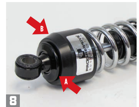
8 A look at the fully assembled shock with the spring retainer clip (arrow A) and top cap (arrow B) in place.
