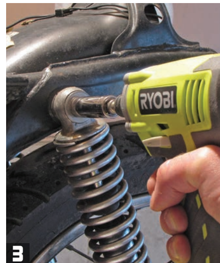
3 Remove the old shocks using a 14mm socket or impact driver and save original hardware. Penetrating oil may be needed to loosen the nuts and bolts.
