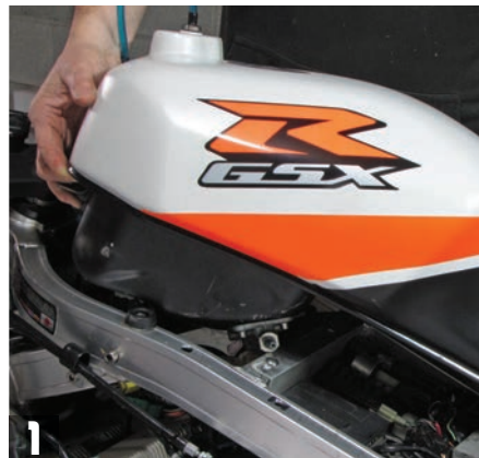
1 Remove tank and seat to allow access to the original clipped-front turn signal wires. Signal relay on this custom GSX-R is also located under the tank.
