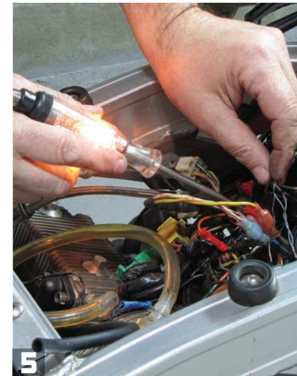
5 Find the hot lead from the signal relay. In this case the wires were clipped and located under the tank. On most bikes, these will be at the original signal location.
