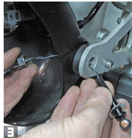
3 Replace the original headlight mounting bolts with Kuryakyn M8 x 40mm threaded studs. Run the Bullet Atto turn signal wires through these bolts and down to the original signal wires under the tank.
