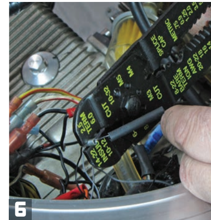
6 Use the provided tin sleeves to connect the new Atto signal wires to the original wires. Use the provided heat-shrink sleeves to seal all connections.
