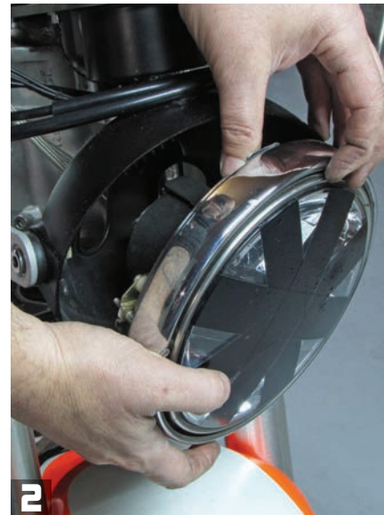
2 Remove the headlight from headlight bucket.
