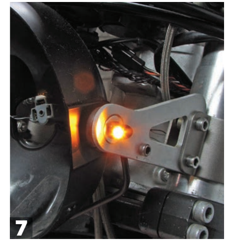
7 Mount the new Bullet Atto turn signals to the M8 x 40mm threaded studs and test the turn signals.
