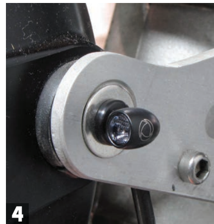
4 Attach the new turn signals to the headlight mounting bracket. The original mounting hardware was much bigger than the new threaded studs we're using, so a flat washer was needed to secure the connection.
