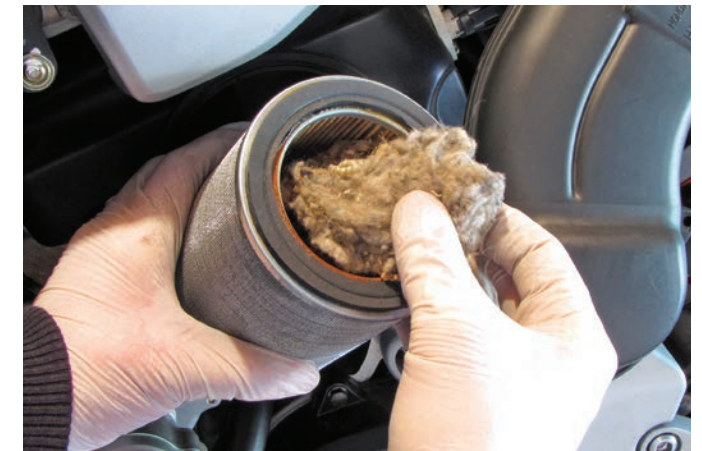
Critters love to find their way into air cleaners or any inviting areas that may provide shelter. Check for nesting and evict these unwanted guests as often as possible.
