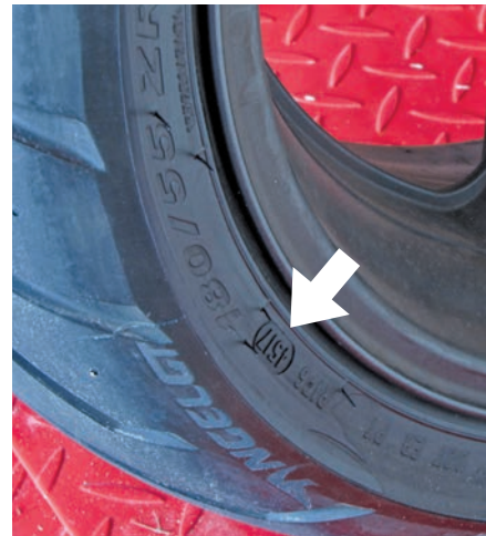
New set of rubber getting scrubbed in. The manufacture date, 4517 (arrow) lets me know these tires were made the 45th day of 2117.
