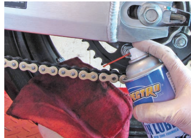
After cleaning your chain, reapply a quality lube like Spectro Z clean chain lube. O- and X-ring chains don't require as much lube as a standard chain, so if running modern links, wipe off any excess with a rag.
