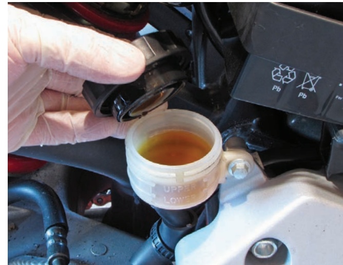
Give your brake fluid, front and rear, a level check and top off if needed. Refer to your owners manual for fluid specs.
