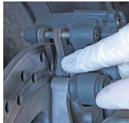
Its easy to see, even without removing the caliper, there's plenty of meat left on these pads. They don't need to be replaced just yet.
